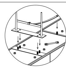
NOW PLACE THE BODY OF MEDIA CONSOLE UPSIDE DOWN WITH THE HELP OF AT LEAST 4 - 5 PEOPLE ON A CLEAN SURFACE. NOW TAKE THE SCREWED LEGS AND ROD AND PLACE THEM IN UPSIDE DOWN POSITION ON THE MEDIA SUCH AS THREADED PORTION OF MEDIA MATCHES WITH THE HOLES IN THE IRON LEGS. NOW SCREW THEM FIRMLY WITH THE GIVEN HARDWARE AS SHOWN IN THE ABOVE IMAGE. NOW KEEP THE PIECE IN THE UPRIGHT POSITION.
