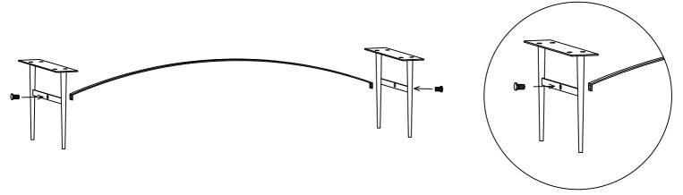
FIRST OF ALL TAKE THE GIVEN LEGS AND THE CONNECTING ROD AND MATCH THE HOLES AS SHOWN IN THE ABOVE IMAGE. NOW WITH THE GIVEN HARDWARE SCREW THE CONNECTING ROD TIGHTLY WITH THE LEGS.
